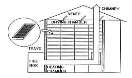
Figure 3: A typical tray drier
